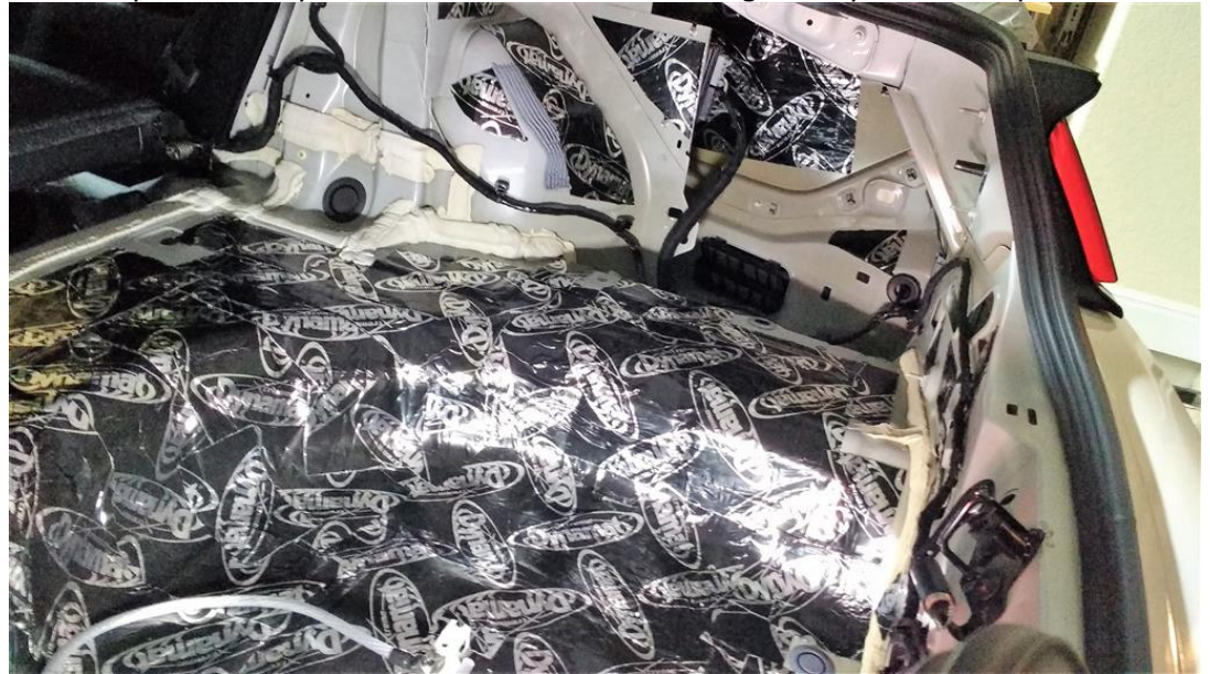
Smaller pieces of Dynamat installed where I thought they would help.
